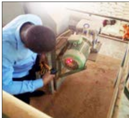
Measuring the speed (rpm) of the motors using digital tachometer
