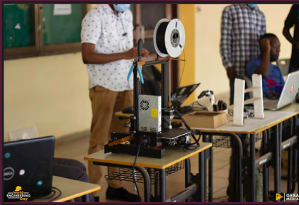
An FDM 3D printer with polymer filament
