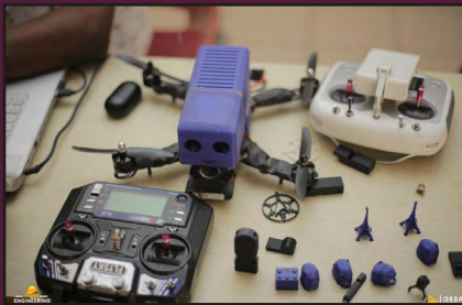
A surveying drone with 3D printed case
